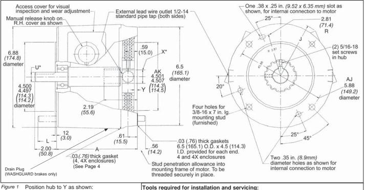
Figure 1 Position hub to Y as shown: Y=.32" (8.1mm) for 1 & 2 disc (1.5 - 15 lb-ft) Y=.19" (4.8mm) for 3 disc (20 & 25 lb-ft)
